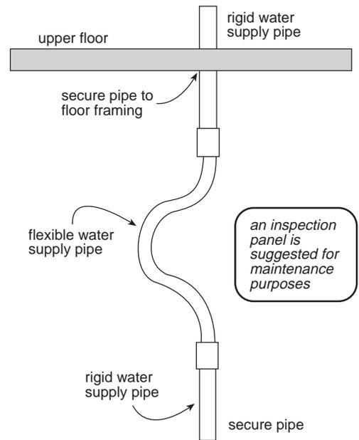
Using a combination of flexible water supply pipe and rigid pipe to allow for needed settling in second-story plumbing.
